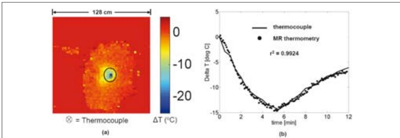
Fig. 2 Comparison of MR-thermometry measurements with MRI-compatible thermocouple
